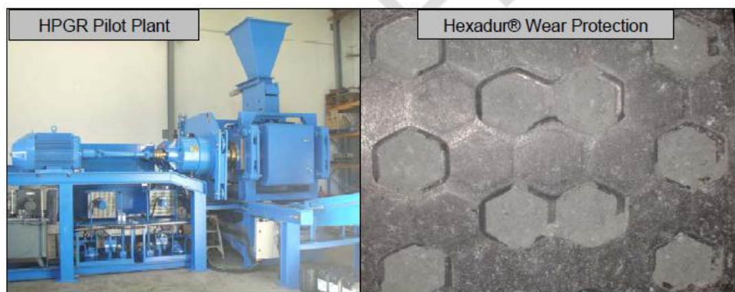
Figure 1: Main view of the HPGR pilot plant and Hexadur® wear surface.
